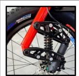
**Double front disc brake** (1 per weel) diameter 160 mm Symmetric double piston each break
